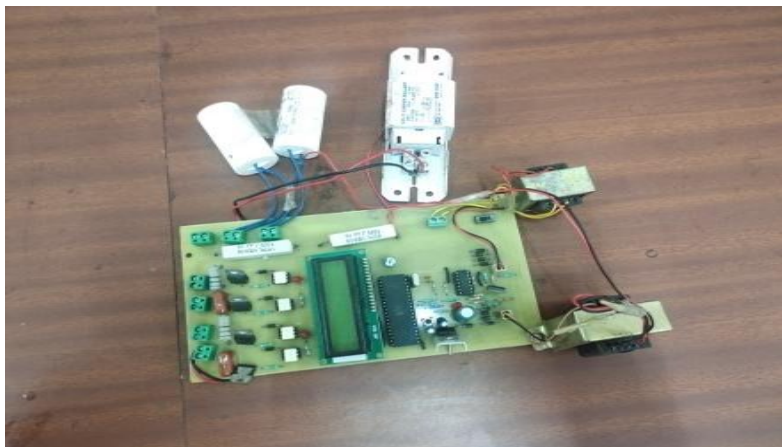
Figure B.6.2.4.TCR /TSR Based Reactive Power Control
