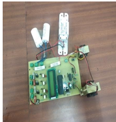
TCR/TSR Based Reactive Power Control
