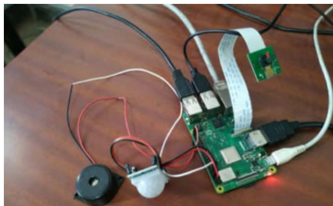
Figure B.6.2.5: Live Model of Smart Intrusion Detection System for Home Security
