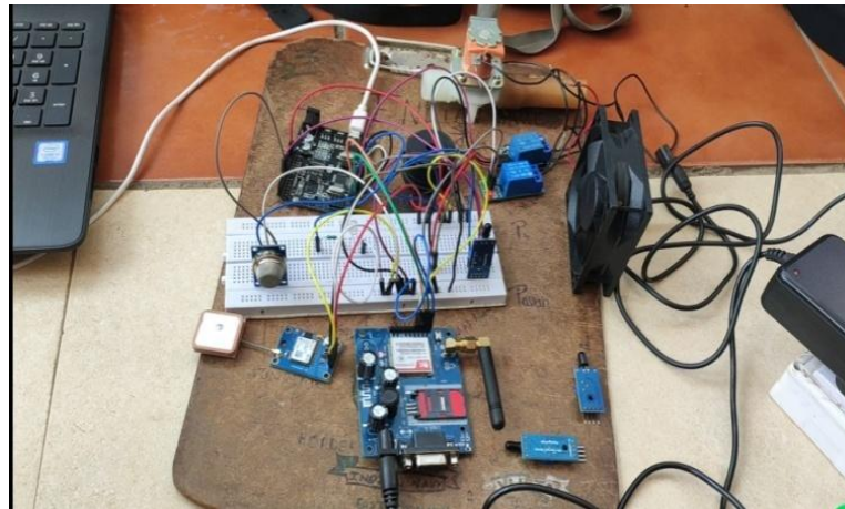
Figure B.6.2.2: Live Model of IoT Based gas leakage and fire alert system
