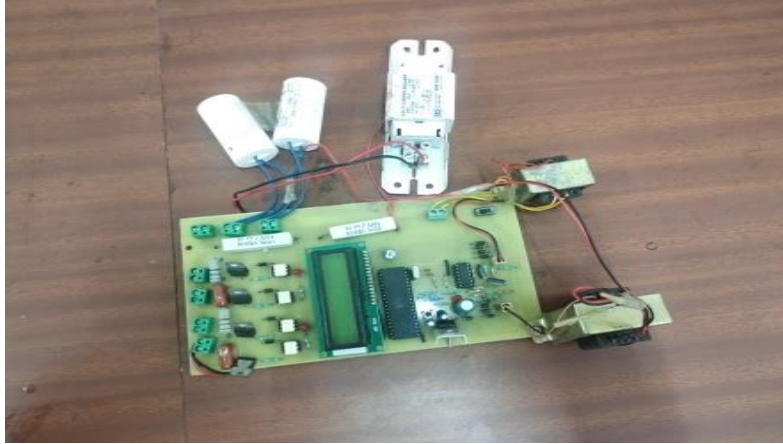
Figure B.6.2.d.TCR /TSR Based Reactive Power Control
