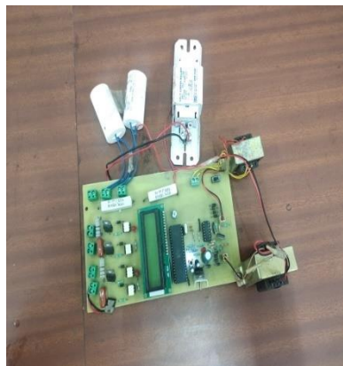
TCR/TSR Based Reactive Power Control
